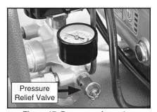
Figure 17. Pressure safety valve.
